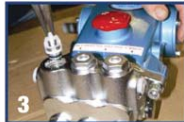
Grasp Spring Retainer by tab at the top with pliers and remove from valve chamber. Check internals of valve for any damage to floating disc or Valve Seat. Replace if necessary
