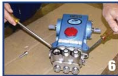
Separate Manifold Head from crankcase by turning the shaft, insert 2 screwdrivers in gap and pry Manifold Head forward until it comes off
