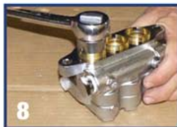
Remove Seal Case from each seal chamber. Remove O-Ring from outside diameter of Seal Case and discard. Be careful not to damage the brass case.
