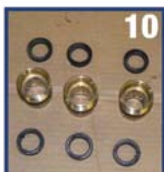
Remove pump from vice and place manifold head in vice. Remove Lo- Pressure Seal from manifold head and discard.
