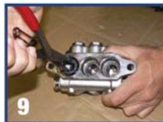
Remove Hi-Pressure Seal from manifold head and discard
