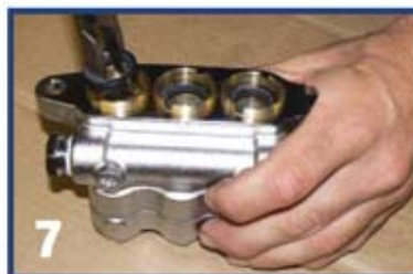
Remove pump from vice and place manifold head in vice. Remove Lo- Pressure Seal from manifold head and discard.
