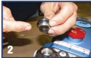
Examine the O-Ring under the Valve Plug for cuts or distortion and replace if worn. Do not lubricate this O-Ring when re-installing
