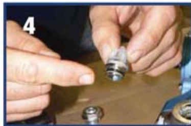
Examine the Valve O-Ring for cuts or distortion and replace if worn. Lubricate the new O-Rings before installing on the manifold
