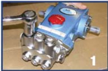
Remove the hex Valve Plugs (top discharge, bottom inlet)
